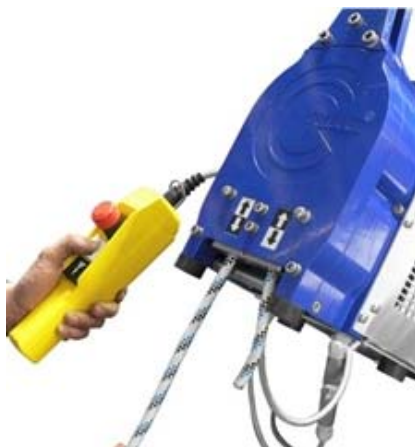
Figure 11: Rope insertion at a standard G-smartrac 300 vario
